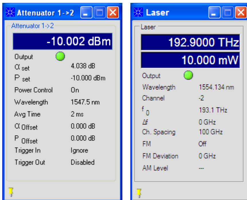
Figure 37 Viewing the measurement on a single channel attenuator/power meter (left) or tunable laser (right)
